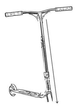
**7-**Close the clamp using the allen tool, do not overtighten the clamp.
